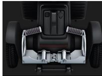
**Stabilizer:** This integration of stabilizer and independent suspension provides unmatched stability, especially in tight turns.
