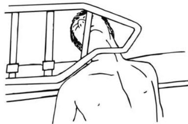
***Entrapment between the end of the rail and the side edge of the head board or foot board***
