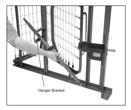
4. Place the foot spring standing up on the floor on its side. Slide Hi/Low shaft through hanger bracket.
